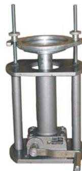
**ESPECIFICAÇÃO****EXTRATOR PARA MOLDE MARSHALL HIDRÁULICO****(ENSAIOS MARSHALL PARA MISTURAS BETUMINOSAS)**
